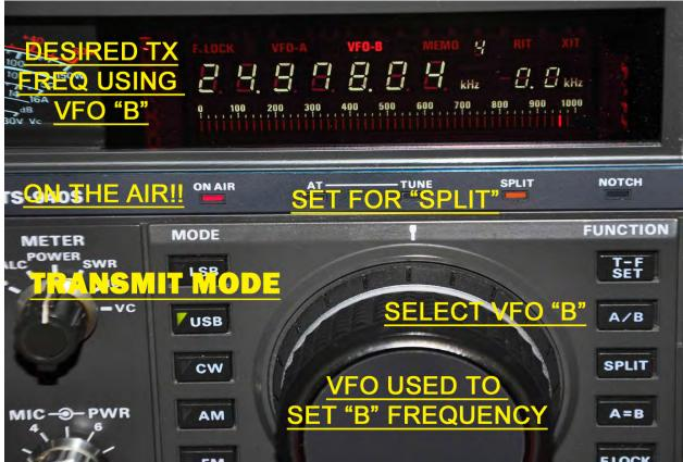
The most desirable set up, however, is to have what is called a "sub-receiver." That gives you the capability to transmit on one frequency, to receive on that same frequency, and <u>at the same time</u> to receive on another frequency. We will talk more about a sub receiver's advantages in a minute.
